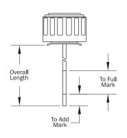
Dipsticks can be fitted to the FBA and FBAP series. Please supply drawing with lengths shown above. Dipsticks will be marked full and add.
