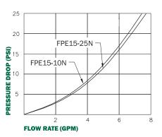
Clean element pressure drop using 150 SSU oil at 100  $^{\circ}\text{F}.$
